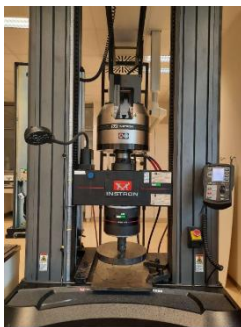
Tensile compression machine load cell (credit HIDRIA).
